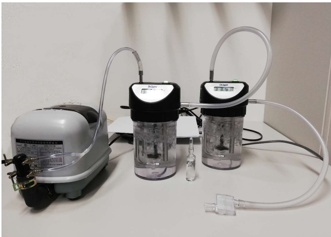
Figure 6: Experimental setup for the conduction of the accuracy study for breath acetone measuring devices. The membrane pump is visible on the left side, the two simulators operated in series are located to the right of it. The test gas is delivered to the Ketoscan breathalyzer through the hose seen in the foreground. The droplet trap at the end of tube was not used; instead the mouth pieces of the breathalyzers were exchanged frequently.
